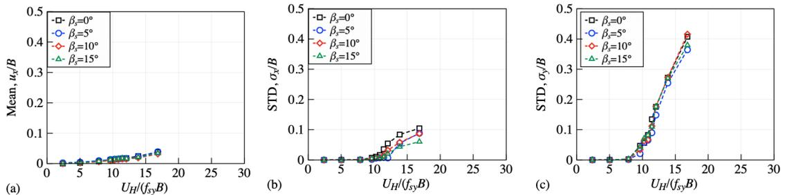
Fig. 12 Effects of the sideward inclination on wind-induced responses under low-turbulent flow:
