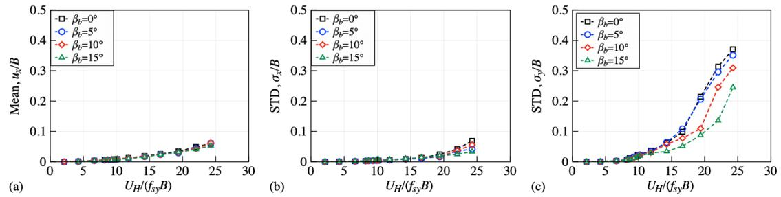
Fig. 11 Effects of the backward inclination on wind-induced responses under boundary layer flow:
