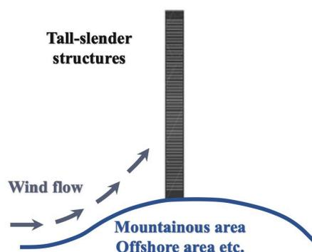
Fig. 2 Sketch of a vertical prism subjecting to pitching wind flow
