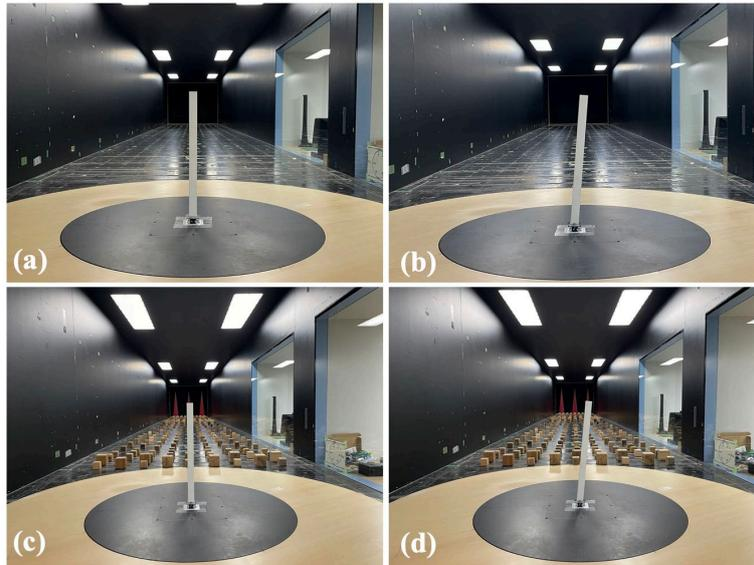
Fig. 6 Experimental model installed in the wind tunnel in low turbulent flow and urban flow: (a) LTF\_Straight ( $\beta = 0^\circ$ ); (b) LTF\_Sideward Inclined model ( $\beta_s = 5^\circ$ ); (c) BLF\_Straight ( $\beta = 0^\circ$ ); (d) BLF\_Inclined ( $\beta_s = 5^\circ$ ).
