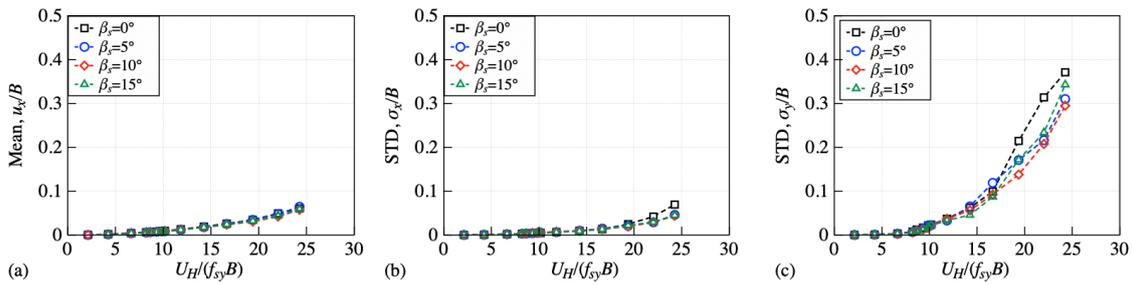
Fig. 13 Effects of the sideward inclination on wind-induced responses under boundary layer flow:
