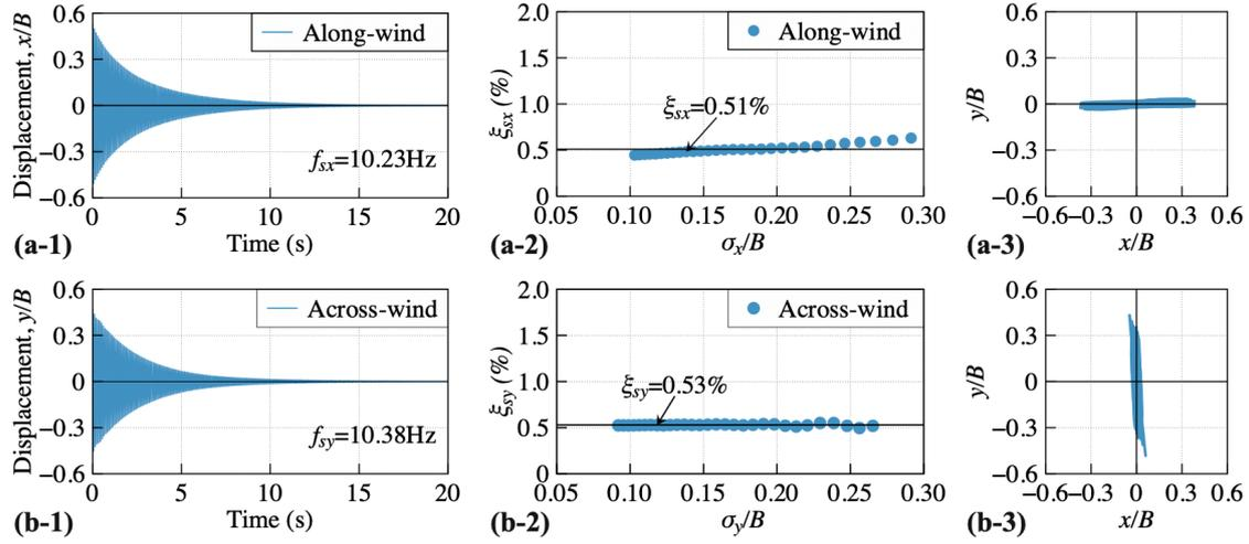
Fig. 3 Free-vibration tests on rocking model high-rise building models with aspect ratio 16 (a-1) Free vibration decay of the along-wind direction; (a-2) Structural damping ratio of the along-wind direction; (a-3) Phase-plane trajectory; (b-1) Free vibration decay of the across-wind direction; (b-2) Structural damping ratio of the across-wind direction; (b-3) Phase-plane trajectory.
