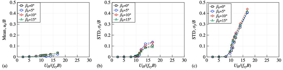
Fig. 10 Effects of the backward inclination on wind-induced responses under low-turbulent flow:
