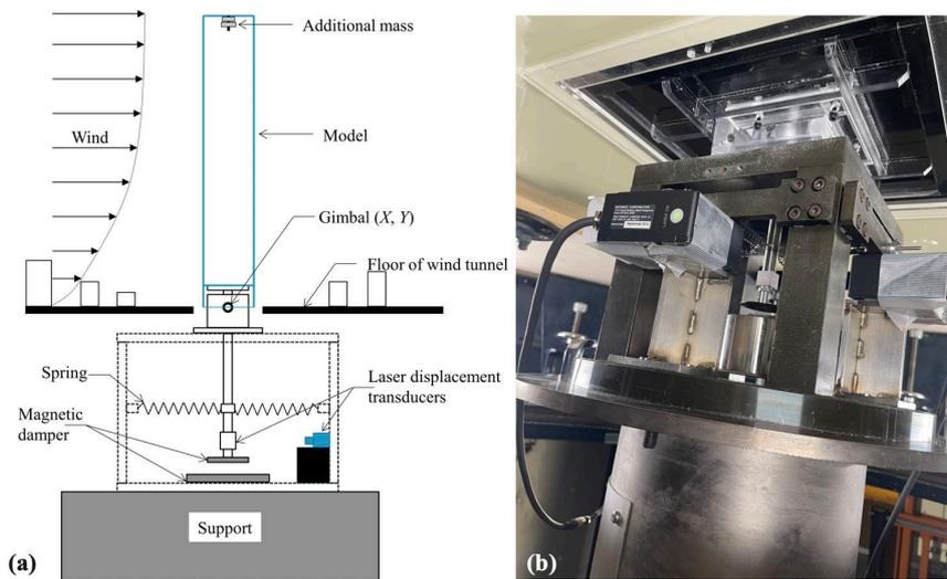
Fig. 2 Equipment of the rocking vibration model tests:
