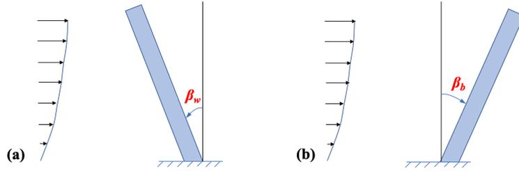
Fig. 7 Illustration of the windward and backward inclinations: (a) windward; (b) backward.
